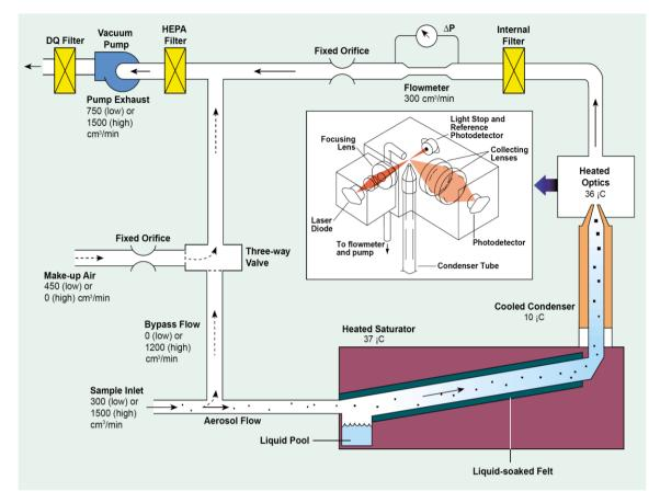
Figure 3. Schematic diagram of the operating principle of the condensation particle counter. [TSI website]
