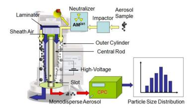
Figure 5. Schematic diagram of a Scanning Mobility Particle Sizer (SMPS) [13].
