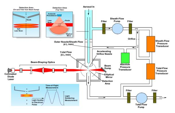
Figure 6. Schematic diagram of aerodynamic particle size measuring equipment [TSI website].
