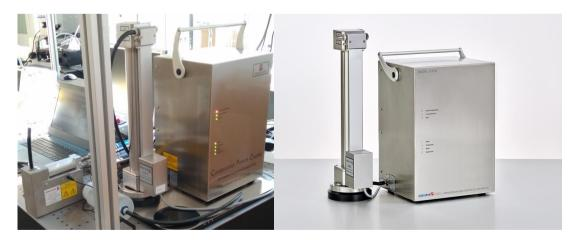
Figure 9. The GRIMM Scanning Mobility Particle Sizer (SMPS)
