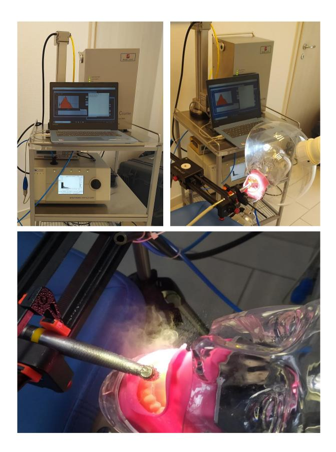
Figure 11. The three measuring instruments and the plastic phantom head during aerosol formation in the dental office
