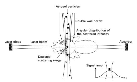
Figure 1. Light scattering on individual aerosol particles, the dashed line shows the spatial distribution of the intensity of the scattered light on a 1  $\mu$ m particle with a refractive index of 1.3 in the case of red laser light.
