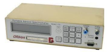
Figure 7. The GRIMM 1.109 optical particle counter.
