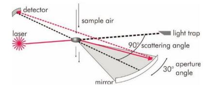
Figure 2. Schematic drawing of the principle of operation of optical particle counters.
