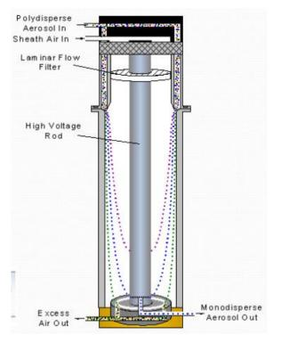
Figure 4. Schematic diagram of a differential mobility analyzer.
